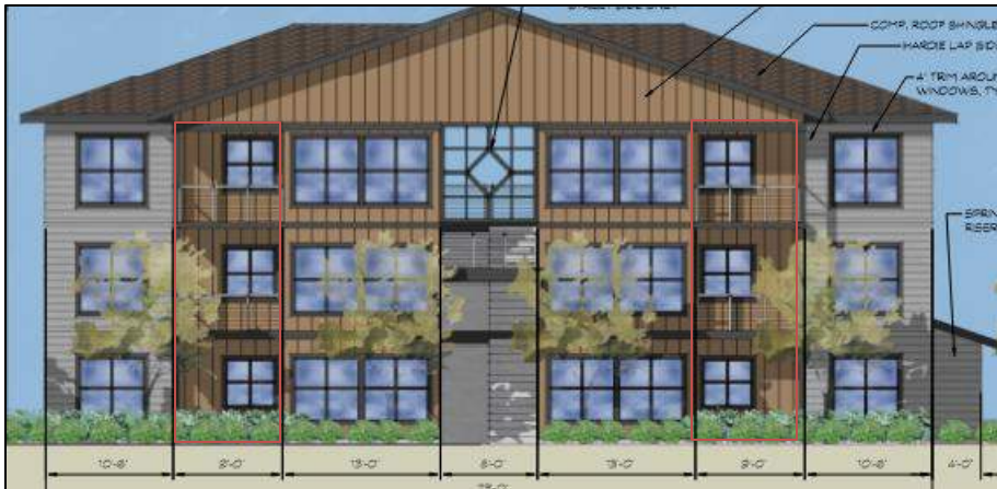
Figure 6 shows the area along the south facade that will need to utilize a different material/color to meet the articulation standard.
